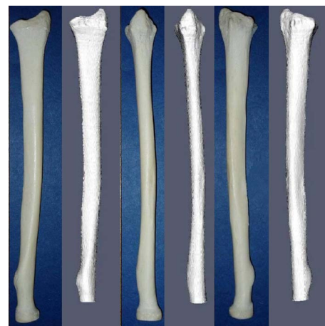
Fig. 13 Actual bone image together with 3D visualization of FE model of bone No. 3; bone in: anterior-posterior, lateral, and posterior-anterior views, starting from the left
