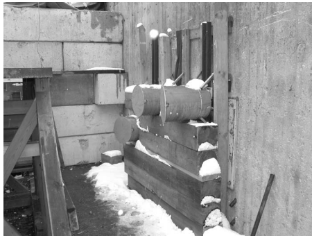
Fig. 6 The three flash X-ray tubes protected from shrapnel and pressure by their aluminum casings
